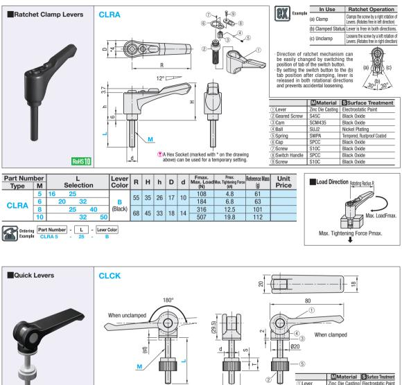
1)Lever Zinc Die Casting Electrostatic Paint ②Thread SS400 Electroless Nickel Plating D Electroless Nickel Plating ③Washer S45C Polyamide (Black) (4) Thrust Washer (5)Clamp Knobs S45C Electroless Nickel Plating
