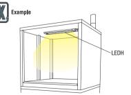
Even in a small device, if it is installed into the ceiling, its wide beam angle enables illumination of the entire area inside the device.
