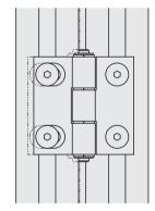
Slotted mounting holes make it possible to adjust right and left positions.
