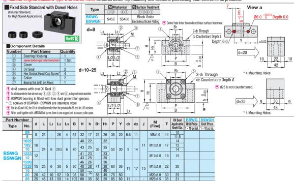
\* Take care in combining No.20 with Ball Screw BSSZ(K)2510, BSSR(K)2510 or BSST2510. The ball screw nut may come in contact with the bottom surfaces.
