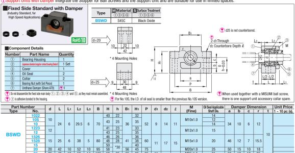
Take care in combining No.20 with Ball Screw BSSZ (K) 2510, BSSR (K) 2510 or BSST2510. The ball screw nut may come in contact with the bottom surfaces
