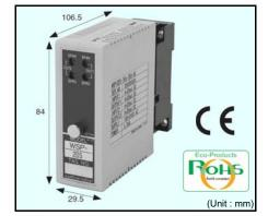
This compact plug-in converter (isolator) has 2 separate input / output circuit. This converter accepts a 2 channel DC voltage or current input and provides optically isolated DC voltage or current output. It amplifies and converts the selected DC input to the selected DC output. And also provides isolation of up to 2000V between the signal input, outputs, and power supply.
