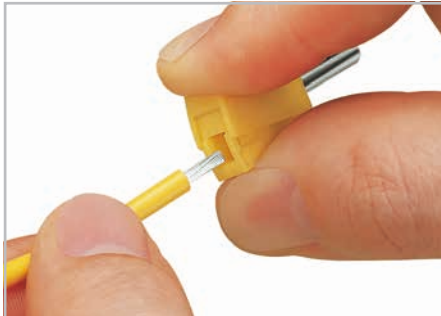
Conductor termination: Press button fully and insert stripped conductor into square entry until it hits backstop and release.
