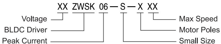
Max Speed: Maximum speed when the motor no-load.(unit: KRPM, For example: 08 mean 8000RPM)
