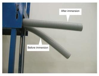
Standard type PVC DUCT cannot be used after immersion in oil, as it has lost flexibility.
