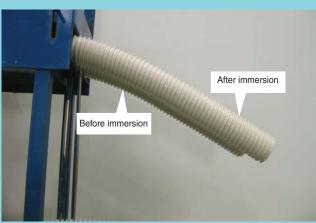
After immersion in oil for a week, no substantial change in flexibility. (Kerosene is used in this test.)
