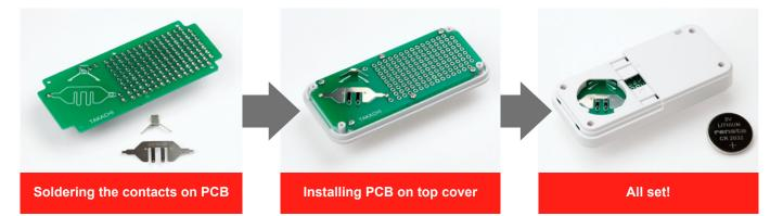
• Exclusive PCB are prepared as the optional parts. See page 44 for the details. Please use the figure of dimensions and screw hole layout on page 8 for your original PCB as well.
