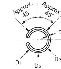
Slot width "C" should be chosen safe from closely contact when spring pins are inserted. (exception: both ends of spring pins)
