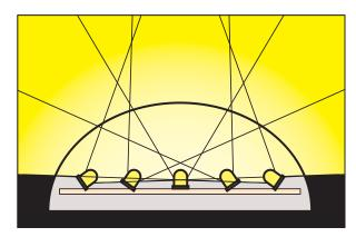
Patlite has created a revolutionary patented lighting design in which multiple LEDs project light across a broad peripheral area, ensuring equal intensity at the sides as well as the front. This design, with its side-projection technology, is a unique achievement in signal light design.
