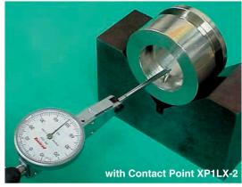
Also makes it possible to measure the parallelism and run-out of grooves on diffrent levels.
