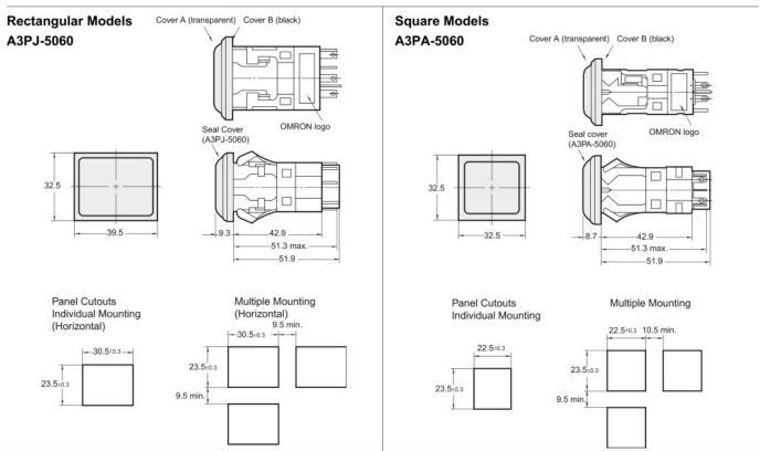
Note: 1. Recommended panel thickness: 1 to 5 mm
