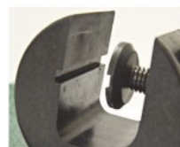
Clamp with grooves to hold calipers securely
