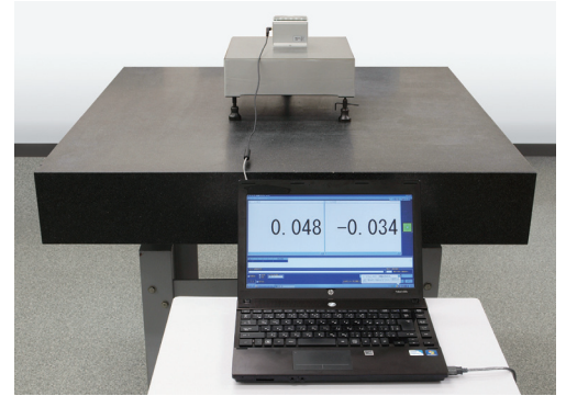
Output from sensors can also be displayed or recorded on PC with dedicated software.
