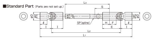
Parts Setup with Key Way and Tap(Designate dimension L1)
