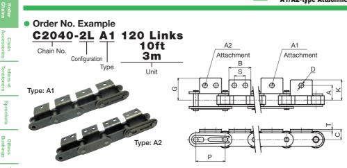
Double pitch roller chains are roller chains for transmission with a double pitch. Small conveyor chains, each part of which is the same as roller chains and which are excellent in rupture strength and wear resistance. The R-type and S-type are available for rollers, and the A1/2 and K1/2 types for chains with attachments.
