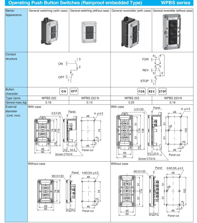
Remark: When you use a contact, b contact, and ab contact independently, please use them with the internal wiring detached.
