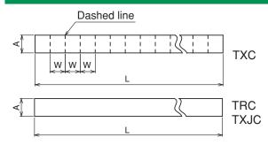
It is possible to set the terminal No. etc. on it. As the partitioning line is printed for TXC type, it is possible to attach it to terminal unit after setting a seal on it, and it is very convenient.
