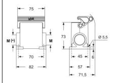
(\*) The surface mounting, high construction housings are supplied with an open threaded entry (\*) and diametrically opposite a closed threaded entry which can be opened by the user if required (with suitable tool).
