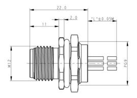
All dimensions in mm. Temperature range: -40 to +85 $^{\circ}$  C.
