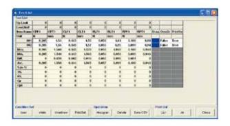
This is application software dedicated to V-103 and V-103A switch feeling. When the optional ROM card V-103 or CF card V-103A is used, measured data/graph data can be loaded to a PC and processed, saved and printed. (The PC and Excel are to be provided by the user.)
