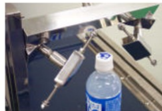
Blowing off of water before shrink wrap packing
