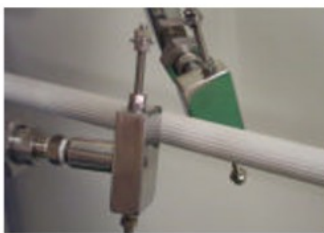
Blowing off water from pipe
